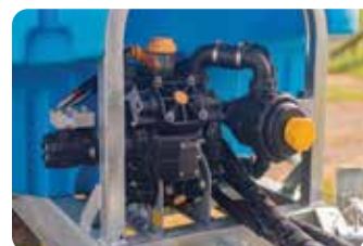
HYDRAULICALLY DRIVEN DIAPHRAGM PUMP
