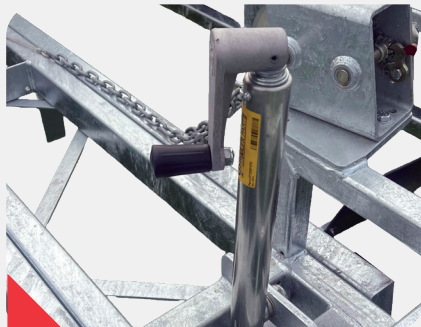
Front to back and sideways levelling system.
