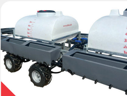
Control taps to fill manifolds from either tank.
