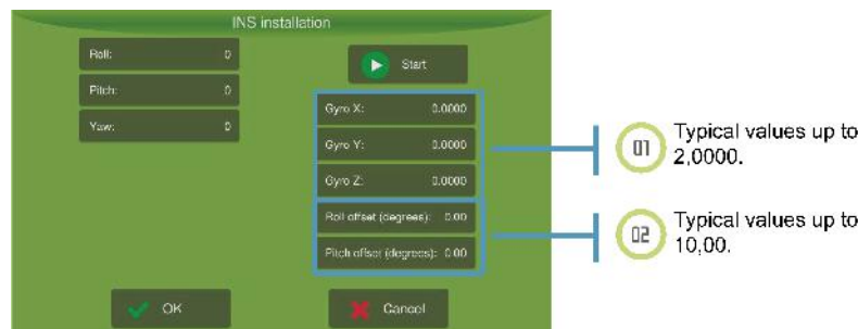
Figure - INS installation
