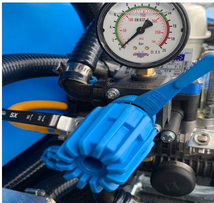
Pressure Adjustment & Gauge MAX 580 PSI
