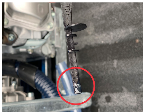
Pump Oil Level (Oil should not exceed max line)
