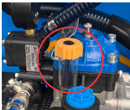
Pump Sight Glass (Oil should not be seen in sight glass when the pump is off)
